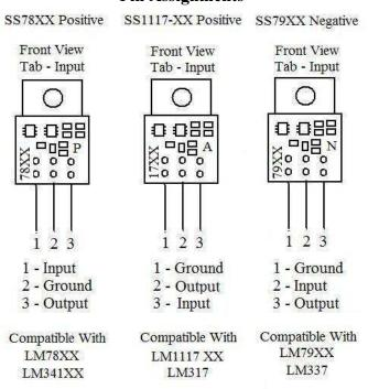
Note that additional circuit modifications are required only when replacing an "adjustable" regulator such as the LM317 / LM337 / LM117-ADJ. When replacing an adjustable regulator, the adjust or ADJ pin must be tied to ground.
