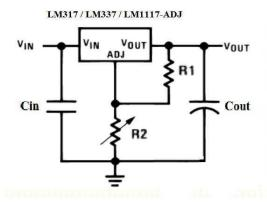
In order to replace an adjustable regulator with one of these discrete devices, R2 must be shorted out, and R1 should be removed. If R1 is not removed, it will result in drawing a steady current of R1/Vout from the regulator. This may or may not be acceptable, depending on the power rating of R1.
