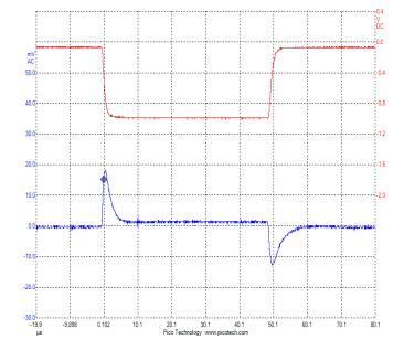
Vo = -15V, Vin = -20V, Load Step = 50mA to 1A Co= 100uF, 10uS / DIV, 10mV/DIV, Load pulse waveform is across 1 $\Omega$ .
