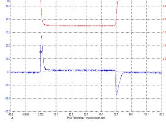
Vo = +15V, Vin = 20V, Load Step = 50mA to 1A Co = 0uF, 10uS / DIV, 10mV/DIV Load pulse waveform is across 1 $\Omega$ .
