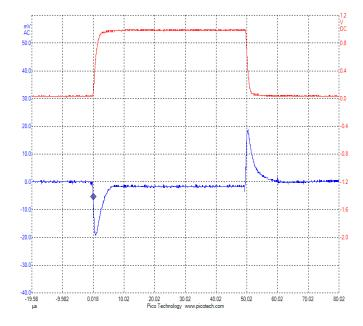
Vo = +15V, Vin = +20V, Load Step = 50mA to 1A Co= 100uF, 10uS / DIV, 10mV/DIV Load pulse waveform is across 1 $\Omega$ .
