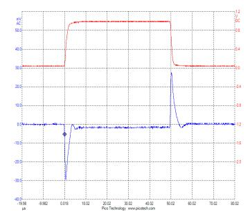
Vo = +15V, Vin = 20V, Load Step = 50mA to 1A Co = 0uF, 10uS / DIV, 10mV/DIV Load pulse waveform is across 1 $\Omega$ .
