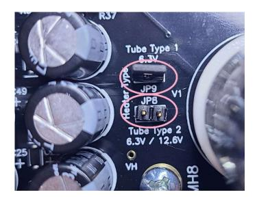
You can roll all types of dual triode tubes into the Gemini. The tube type jumper must be set appropriately depending on which tube type is being used.
